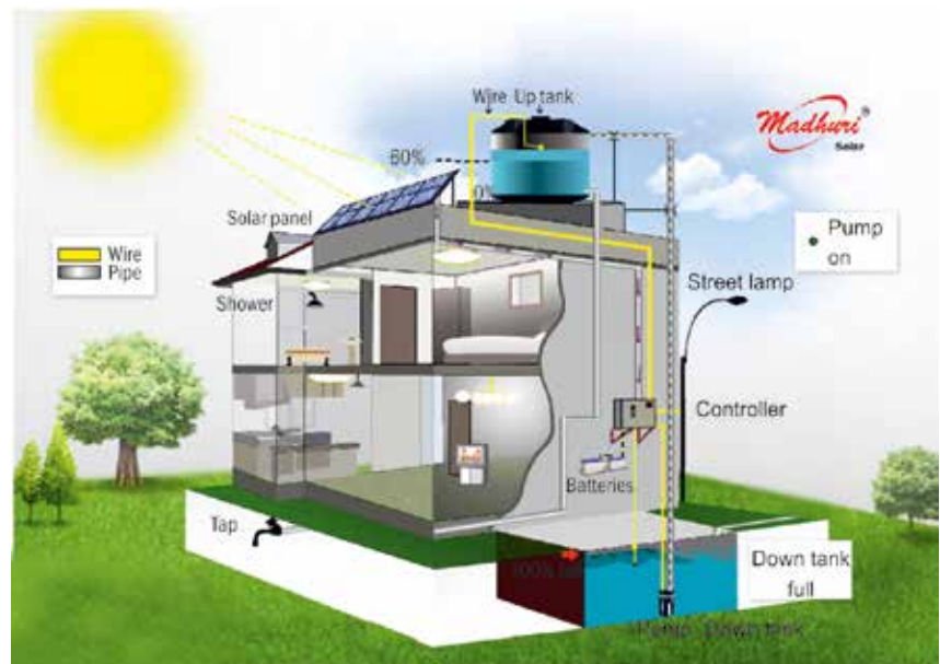
Figure 1: With sunrise the solar water pump gets 'ON' till tank is 100 per cent full
