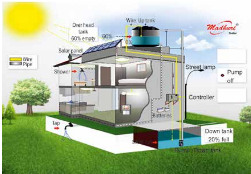
Figure 2: The pump remains 'OFF' till level of tank is reached 60 per cent and after that pump again automatically gets 'ON'
