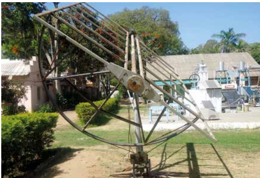
Picture 4: The solar tracker set-up for the direct alignment of the solar panels towards the sun
